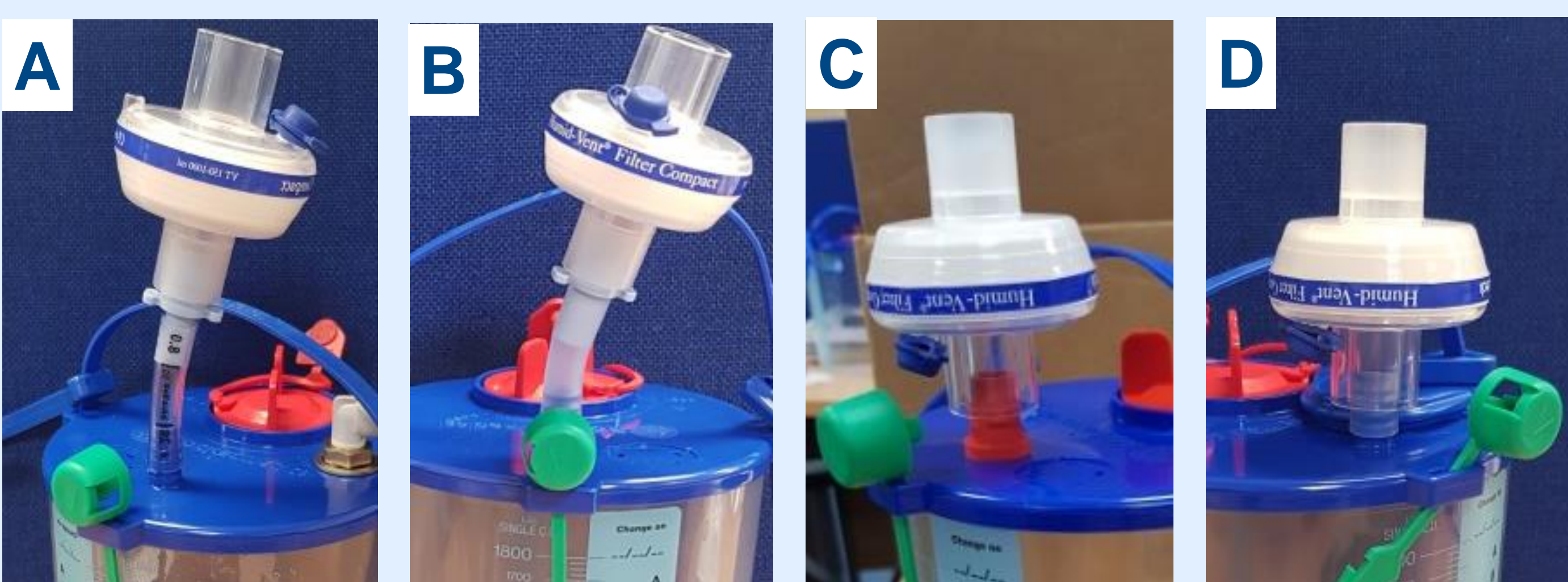
Figure 1: The four design solutions under consideration. Each connects a Teleflex Gibeck Humid-Vent Compact Filter to the outlet of a R54500 Rocket Blue Drainage Bottle System, using A) an endotracheal tube connector and a 5cm segment of endotracheal tubing; B) an endotracheal tube connector and a 5cm segment of chest drain tubing; C) a rubber adapter; D) a 2cm segment of chest drain tubing.
